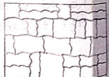
(uncoursed Rubble) (Random Rubble Masonry)
